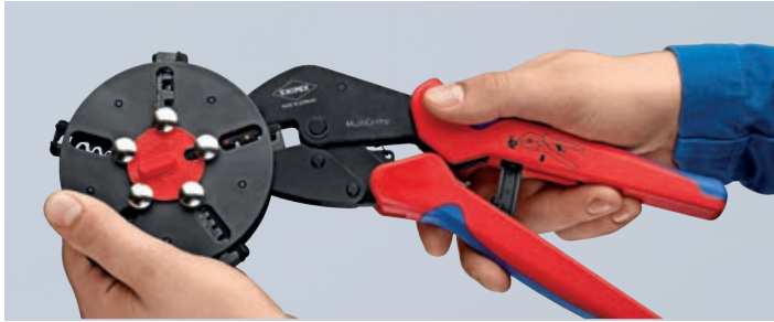
Changing the crimping dies: unlock the magazine position, take out the set of dies which the pliers have been pushed on
