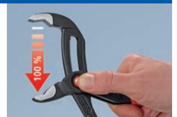
Press the button – open pliers completely
