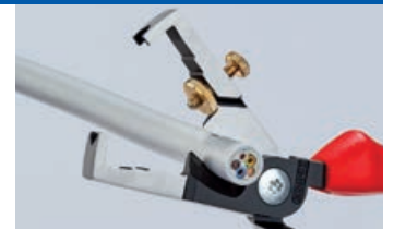
Induction hardened shear blade with precisely ground cutting edges for crushing-free cutting of copper cables up to Ø 15 mm (5 x 2.5 mm 2 )
