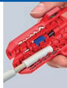
Stripping of the sheath of a NYM cable
