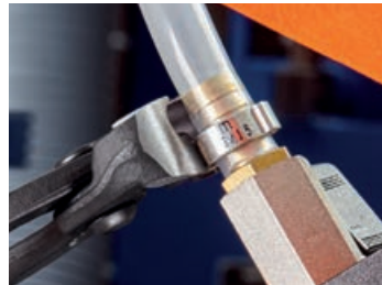
10 98 I220: Sealing the hose connection on central lubrication
