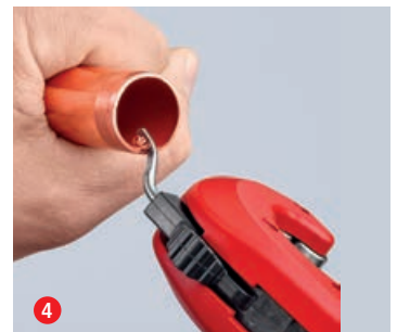
4 And you're done! If necessary, have the edge smoothed out using the fold-out deburring tool – with surprisingly little effort
