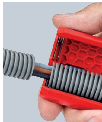
Clean cutting edge with no damage to internal cables as the cut is always at the top of the corrugation
